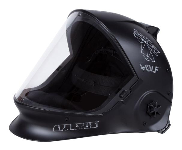
The **SPARTUS**® air supply system has a high level of respiratory protection TH3P thanks to a set of replaceable filters, including a main HEPA filter and an activated carbon pre-filter. The whole system is protected by a spark shield. The connection between the breathing hose and the visor housing provides freedom of movement during work.
